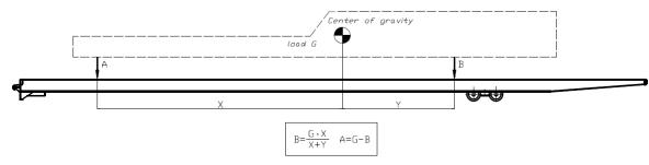
3) Make sare, load center of gravity is in the detemined area
