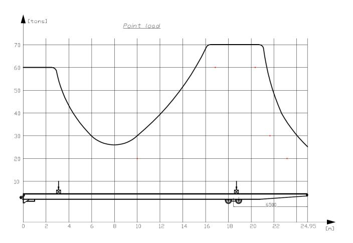
Point loads on the platform to be placed or transferred using transversal supports to the longitudinal beams
