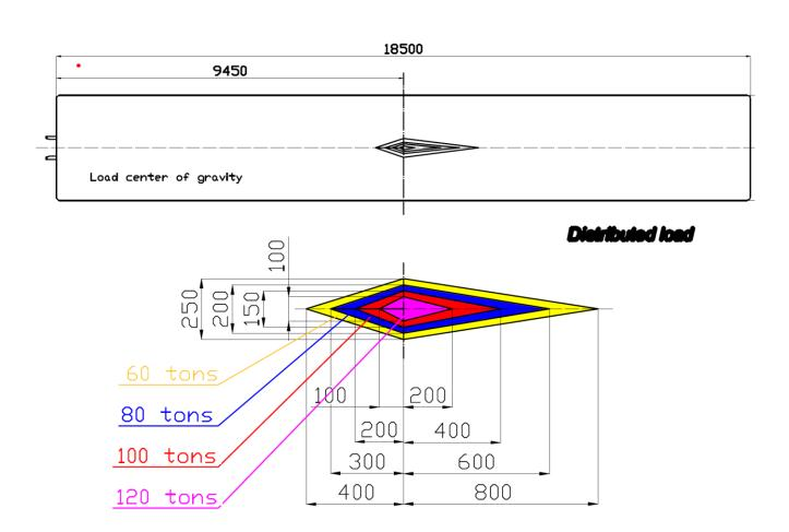
Load center of gravity must be within the areas, corresponding to the load
