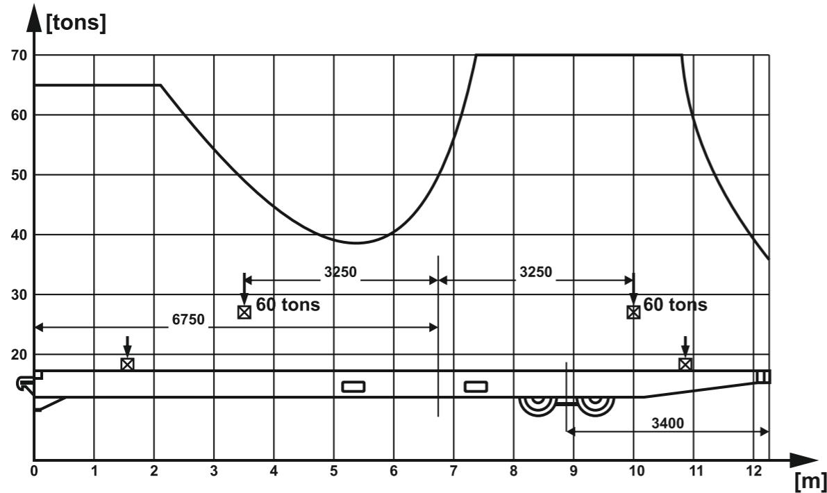
Point loads on the platform to be placed or transferred using transversal supports to the longitudinal beams
