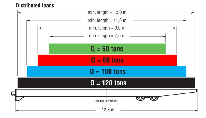
Load center of gravity The center of gravity of the load must be within the respective marked areas 0 --- -Payload up to 120 to Payload up to 100 to Payload up to 80 to 1000 Payload up to 60 to
