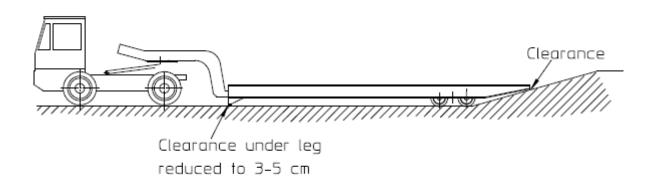
• When the trailer wheels have passed the upper end of the ramp, driver must lift the fifth wheel to maximum height to achieve a sufficient ground clearance under longitudinal beams of the trailer (see sketch below).
