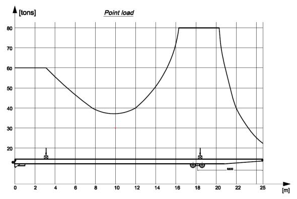
Point loads on the platform to be placed or transferred using transversal supports to the longitudinal beams
