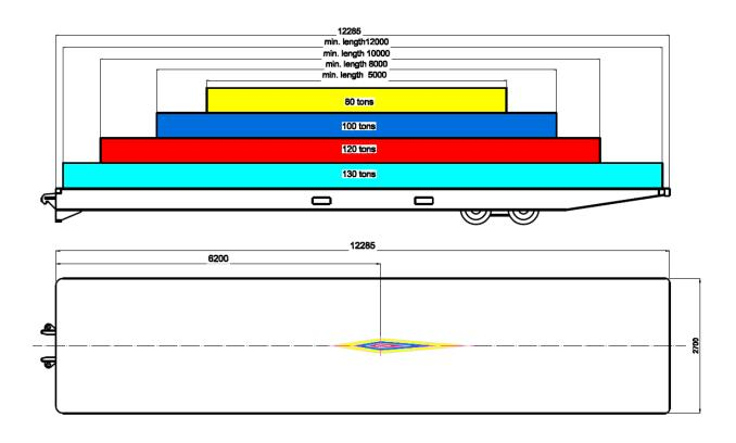
Load center of gravity must be within the areas, corresponding to the load
